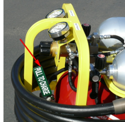
Foam Charge/"Pull to Charge" Valve
